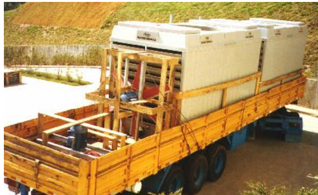
Carreta comum com 2 torres modelo HD-21107 de 250m³/h cada. Standard truck with two "half-assembled" cooling towers for 1100 GPM each.
