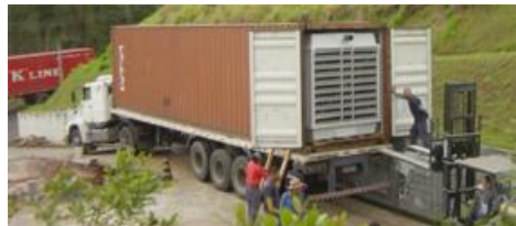
Torre de 200 m³/h em container 40'; 880 GPM cooling tower in 40' container.
