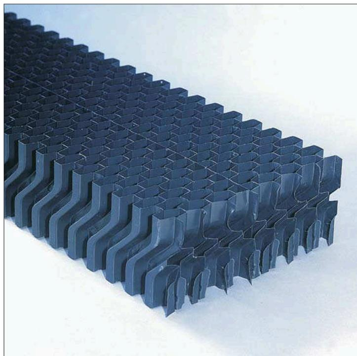
**THE H130 DRIFT ELIMINATOR**, with a geometry based upon 2 changes in the discharge airflow direction, is applied principally in situations of vertical airflow but can also be used for crossflow applications: it is constructed from preformed PVC sheets, subsequently made up into panels.
