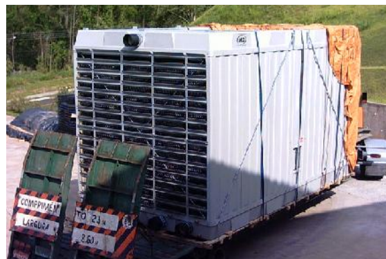
Torre HD-22210-GRT-Semi montada de 500 m³/h; 2200 GPM cooling tower model "half-assembled".
